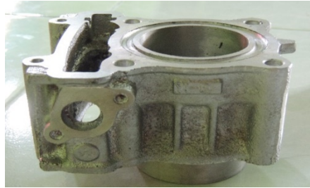
Gambar: 4.16 Hasil finishing blok silinder coran
