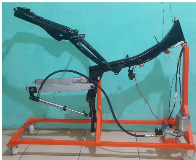
Gambar 4.9 *Prototype* Standar Tengah Hidrolik Sepeda Motor Anti Maling
