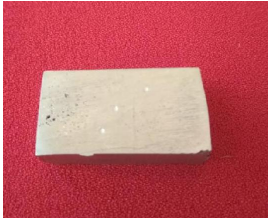
Gambar 3.10 Specimen Standar Uji Kekerasan
