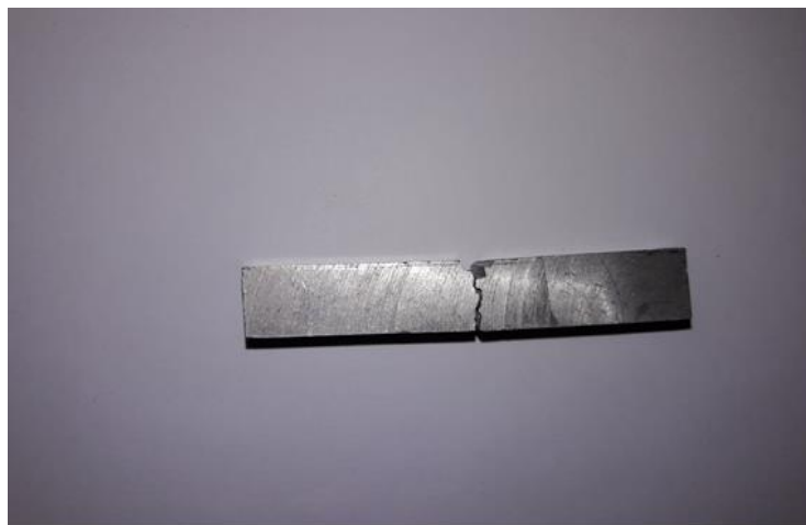
Gambar 3.9 Specimen Standar Uji Impact
