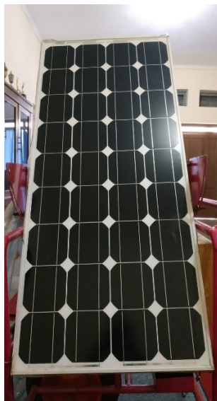
Gambar 3.2. Panel Surya Monocrystalline 100 Wp
