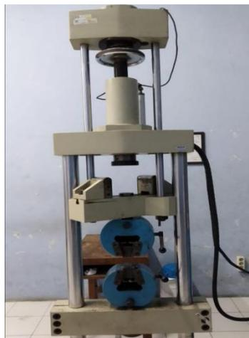
Gambar 3.2 Mesin Uji Tarik tipe controlab/TN 20 MD
