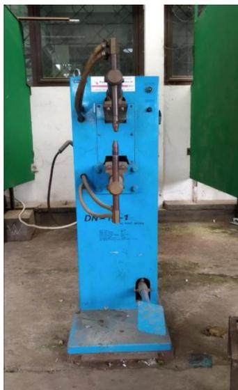
Gambar 3.1 Mesin *spot welding* DN-16-1
