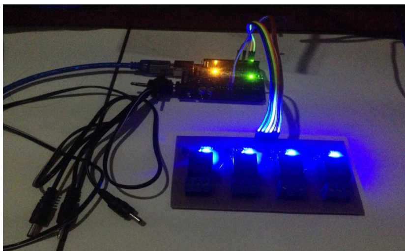
Gambar 4.14 Ujicoba driver relay
