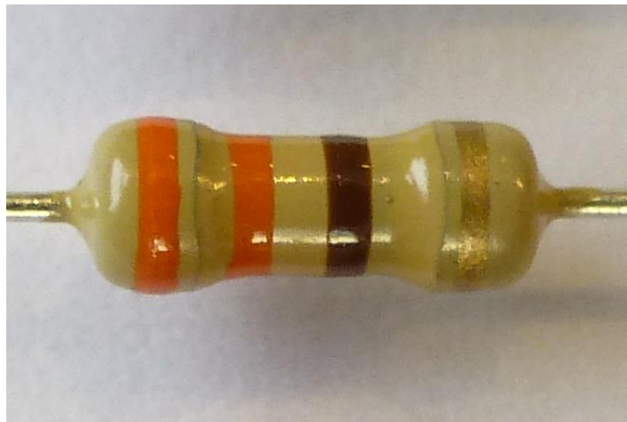
Gambar 2.23 Resistor 330 Ohm( \Omega )
