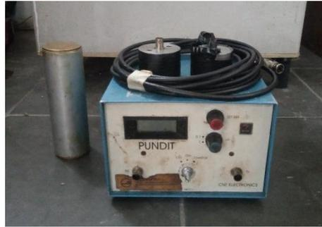
Gambar 3.18. *Ultrasonic Pulse Velocity Test*
