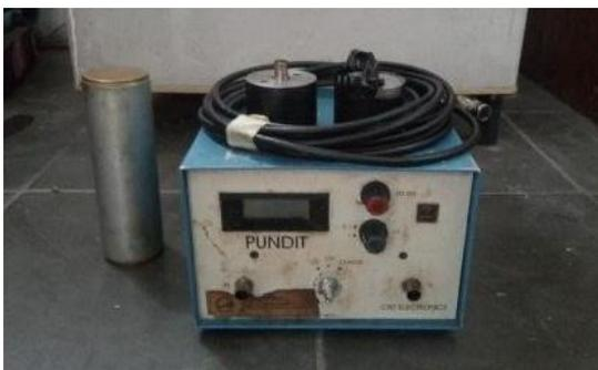
Gambar 4. *Ultrasonic Pulse Velocity Test*
