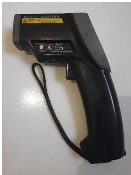
**Gambar 4.8** *Infrared thermometer*
