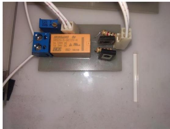
Gambar 3. 10 Rangkaian Driver Motor
