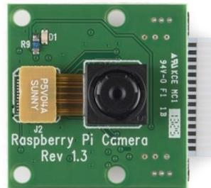
**Gambar 2.7** Modul Kamera *Raspberry Pi* (OV5647)[21]
