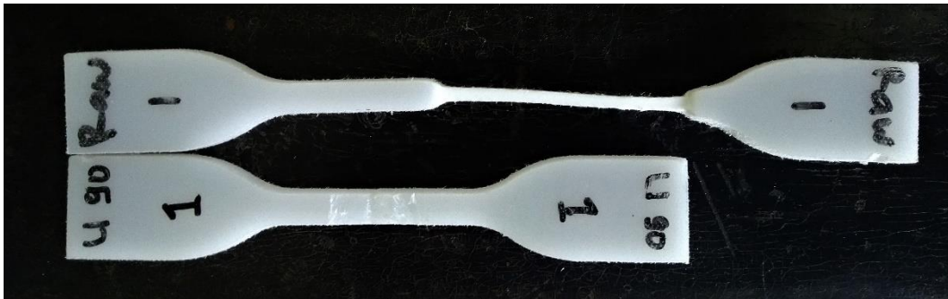
Gambar 4.12 Hasil Uji Tarik Raw Material
