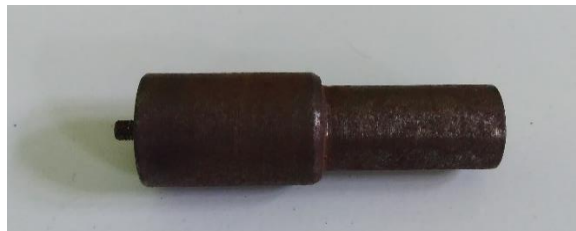
Gambar 3.5 Pin tool silinder ulir 3 mm
