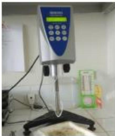
**Gambar 3.9.** Alat Viskometer
