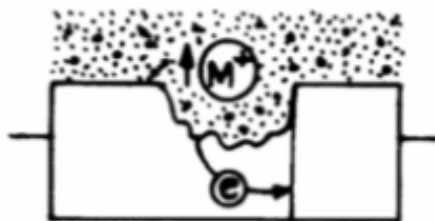
Gambar 7. Galvanic corrosion (Chaturvedi, 2013)
