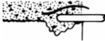
Gambar 5. Crevice corrosion (Chaturvedi, 2013)
