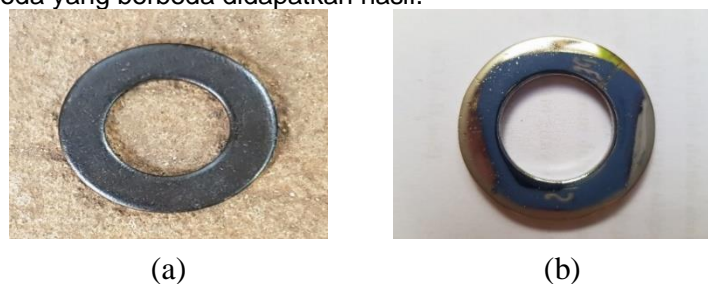
Gambar 4 (a) raw material (b) Ring Plate sesudah proses electroplating .
