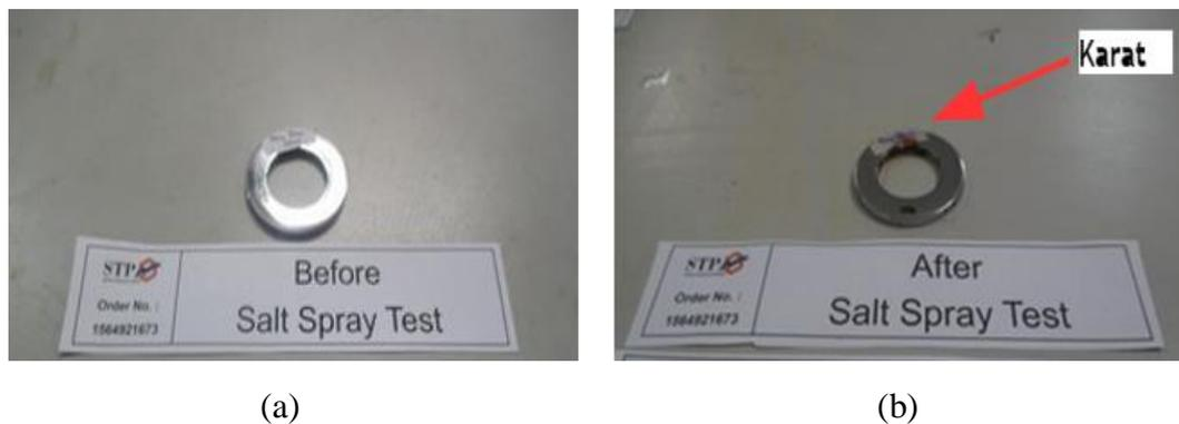
**Gambar 4.9** Spesimen *Ring Plate* Jarak *Throwing* Anoda-Katoda 17,5 cm
