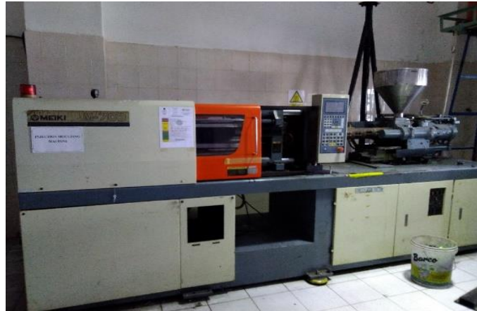
Gambar 2.2 Mesin injection molding .
