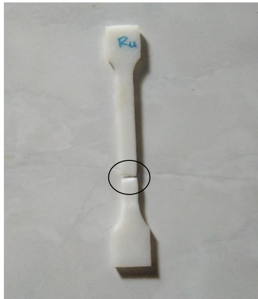
Gambar 4. 15 Patah uji tarik polyamide 6 variasi MC 1%.
