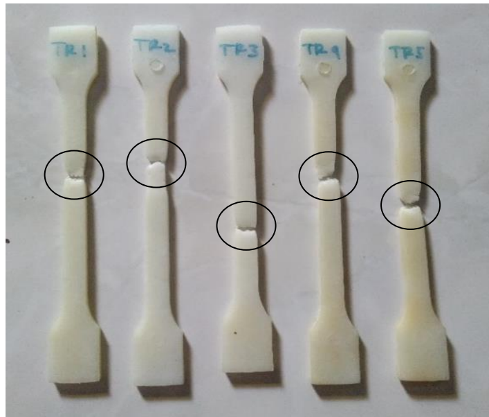
Gambar 4. 17 Patah uji tarik polyamide 6 variasi MC 5,5%.
