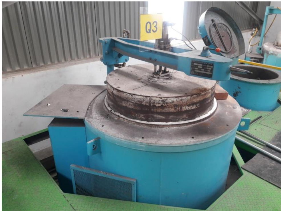
Gambar 3.3 TD Process (Toyota Diffusion Process)
