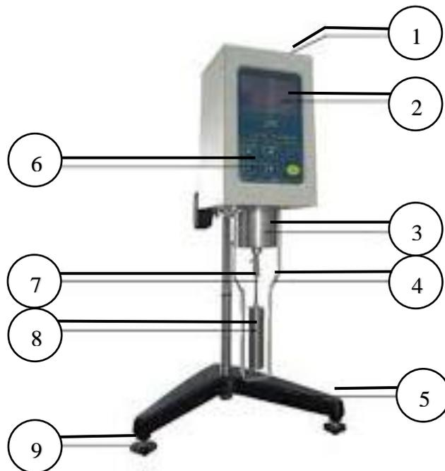
**Gambar 3.8.** Bagian–bagian viskometer NDJ 8S
