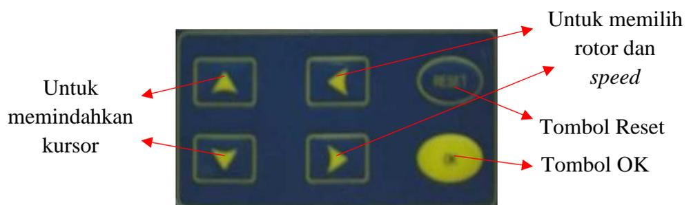
**Gambar 3.11.** Tombol Viskometer
