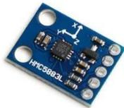
**Gambar 2.4** Sensor Kompas HMC5883L
