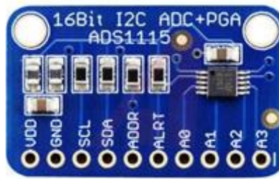
Gambar 2.11 : ADC Adafruit 4 Channel ADS1115
