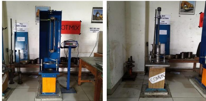
Gambar 3.12 (a) *Automatic Asphalt Compactor* (b) *Manual Asphalt Compactor*
