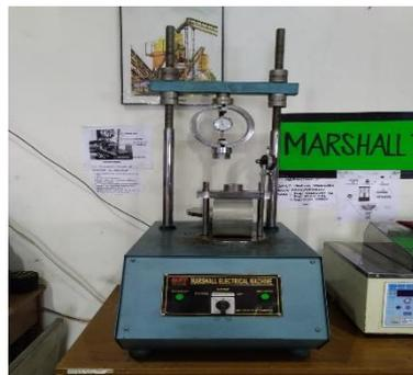
Gambar 3.16 *Marshall Electrical Machine*
