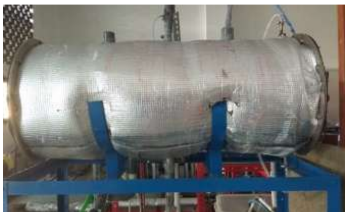
Gambar 3.6. Tangki Solar Water Heater
