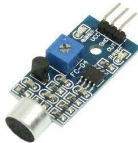
Gambar 2. 7 Sensor Miccondenser[21]
