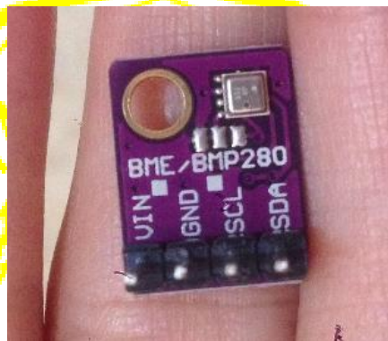
Gambar 3.6 Tampilan Sensor BME280
