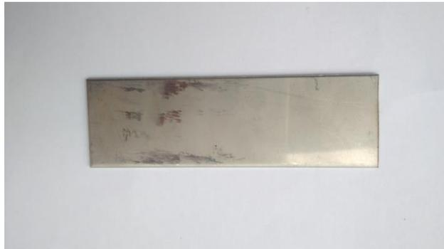
Gambar 3.5 *Stainless Steel* AISI 304 ukuran 80 ml x 25 ml
