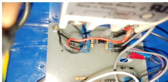
Gambar 3. 5 Rangkaian driver heater
