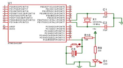
Gambar 2 Rangkaian *Minimum System*
