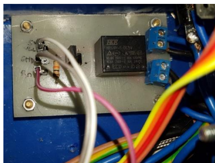
Gambar 3. 8 Rangkaian Driver Valve
