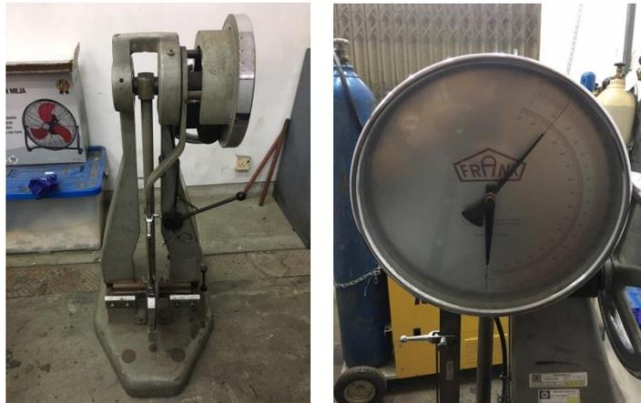
**Gambar 2.8** Mesin uji impact
