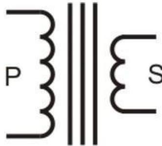
**Gambar 2.4** Simbol *Transformator Step Down*
