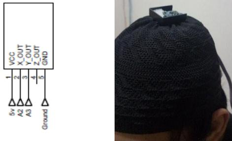
Gambar 4 Modul Accelerometer ADXL335
