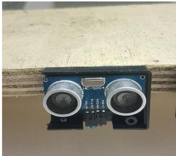
**Gambar 4.3** Peletakan Modul *Ultrasound*
