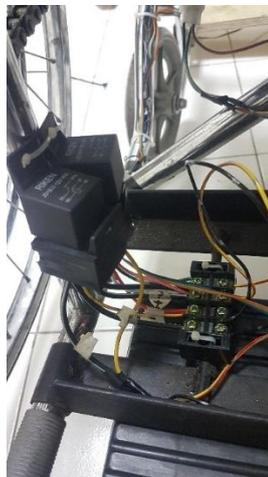
**Gambar 3.8** Rangkaian *Driver* Motor
