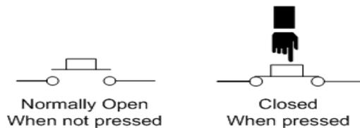
**Gambar 2.4** *Wiring Push Botton*
