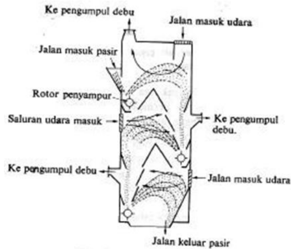
Gambar 2.13 Alat pendingin pasir tegak. (Anonim, 2008)
