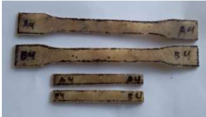
Gambar 3. 13 Hasil Potongan Specimen
