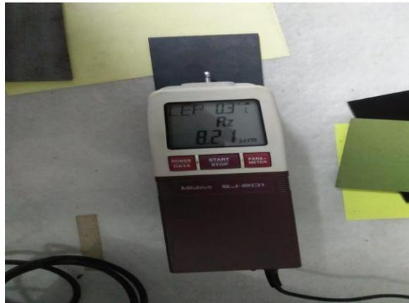
Gambar 2.4 : *Surface Roughness Tester Mitutoyo SJ-201*
