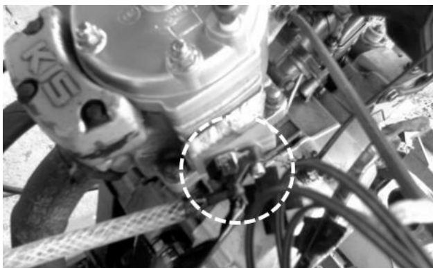
Figure 8. The position of the gasoline injector for low pressure GDI setup
