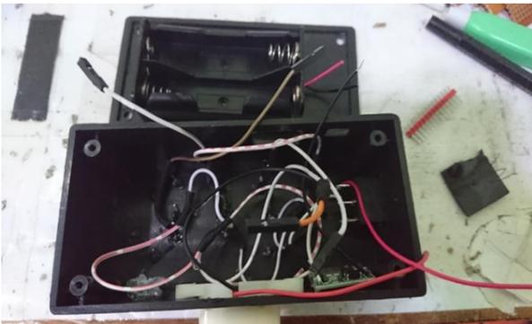
Gambar 3.9 Pemasangan LED Buzzer Didalam Box
