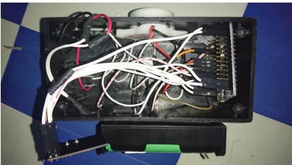
Gambar 3.10 Rangkaian Pada Box Receiver
