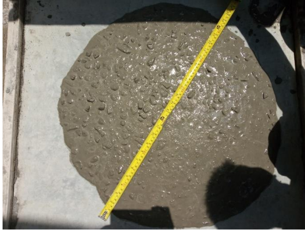
Gambar 4 Pengujian slump flow
