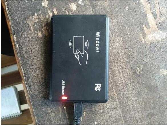
Gambar 4.12 Reader RFID (Radio Frequency Identification)
