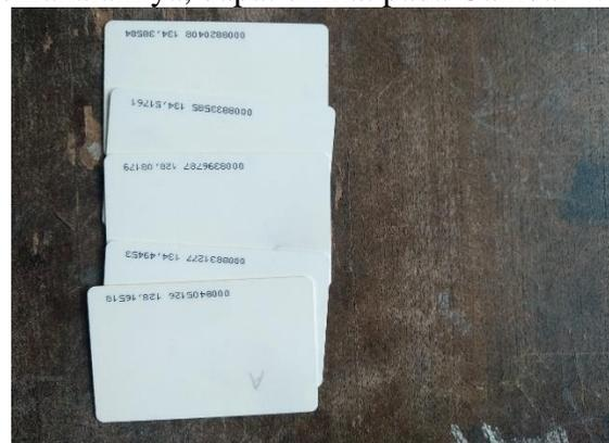
Gambar 4.11 Kartu *RFID* (*Radio Frequency Identification*)
