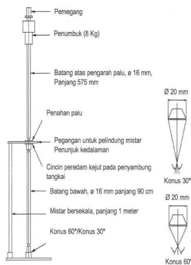
Gambar 2.2 Bagian-bagian alat uji DCP
