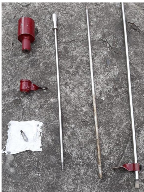
Gambar 3.20 Bagian-bagian alat DCP
