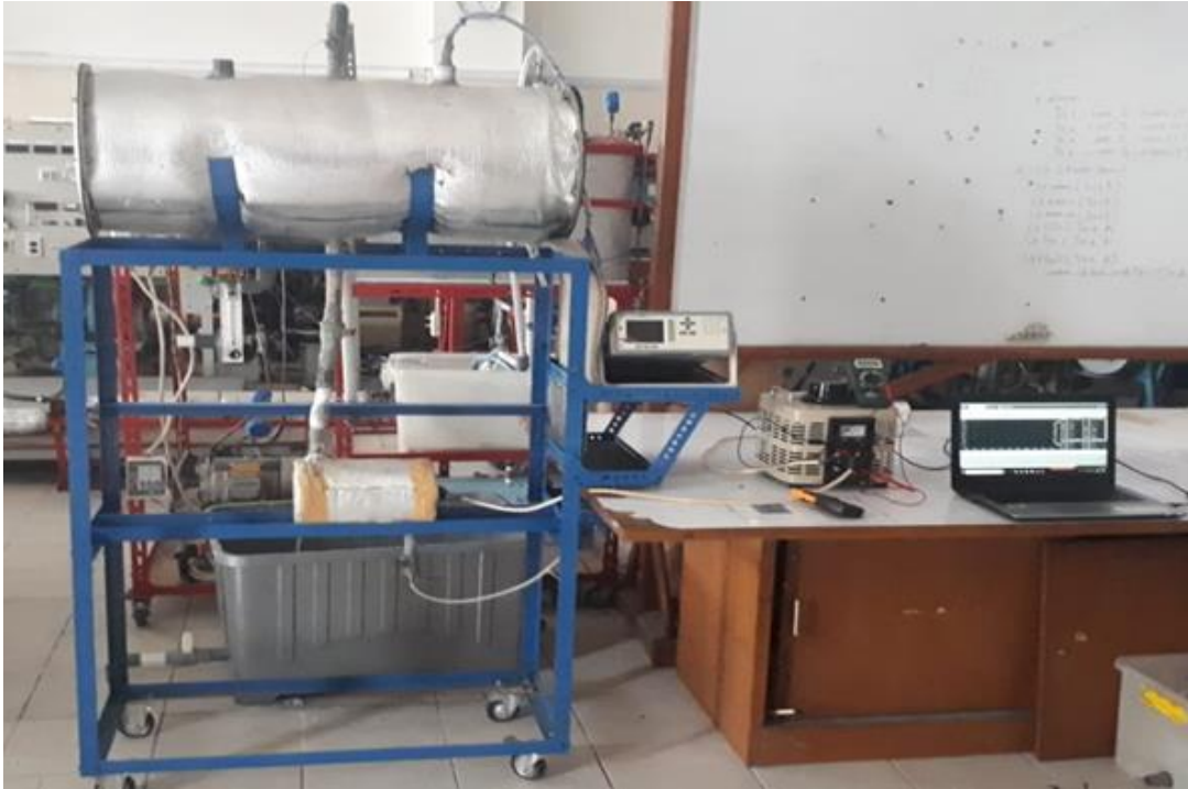
Gambar 3. 4. Alat Penelitian Solar Water Heater
