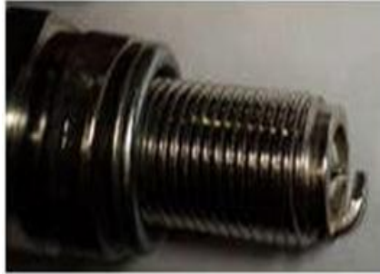
Gambar 3.8. Busi racing Denso Iridium Power
