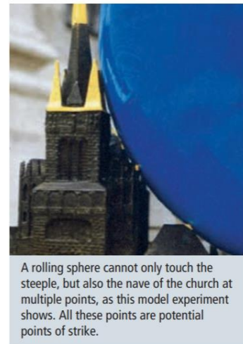
Figure 5.1.1.2 Model of a rolling sphere; source: Prof. Dr. A. Kern, Aachen
